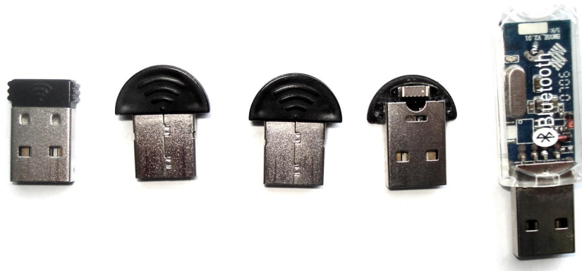
FIGURE 7.3: Photo of purchased Bluetooth USB adapters with incorrect Bluetooth Device Addresses.
